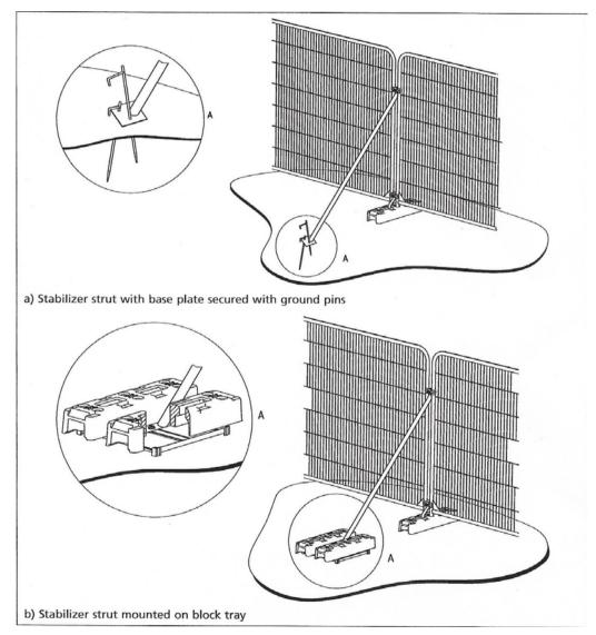
Figure 1. Protective tree fence specification, as per BS 5837.
